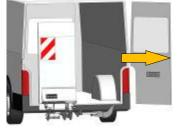
2. Open the right vehicle door to access the control panel or the optional 3-button handheld control.
