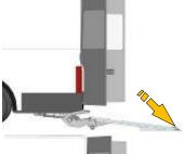
9. Tilt down the tip of the liftgate platform using the control panel (Open/Tilt down) or, if you're standing on the platform, using the foot controls or the optional 3-button handheld control (Tilt up/Tilt down) + (Lower).
