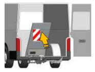
19. Close the liftgate platform using the control panel (Close/Tilt up).
