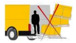
(18) A moveable liftgate may be moved only when the lifting device is in the driving position (see pages 2 and 3. The one exception is when the necessary stability is guaranteed and certified in the inspection record book.
