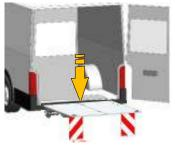
5. Lower the liftgate platform using the control panel (Lower) or, if you're standing on the platform, using the foot controls or the optional handheld control (Lower) so that you can open the left vehicle door.
