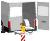
3. Open the liftgate platform using the control panel (Open/Tilt down) or the optional 3-button handheld control (Tilt up/Tilt down) + (Lower).
