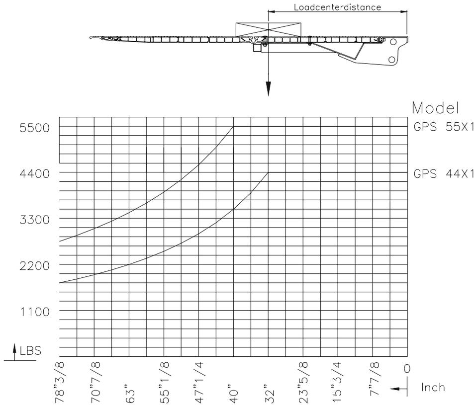
The maximum loading capacity specified in the loading diagram must not be exceeded. The platform may not be used as a bridge plate.
