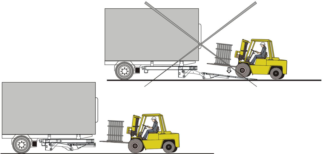
Only when the Slidelift is retracted under the vehicle.
