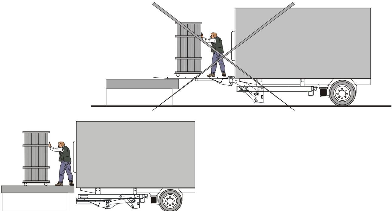
Only when the Slidelift is retracted under the vehicle.
