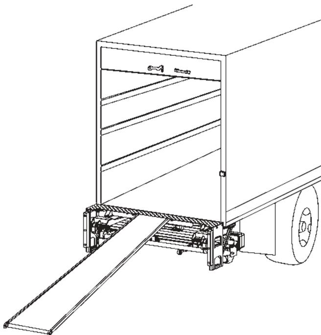
**CAMION ÉQUIPÉ D'UNE RAMPE D'ACCÈS ET D'UN HAYON GPTWR
