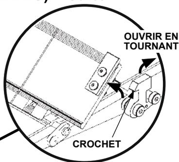
**OUVRIR LES BUTÉES D'ARRÊT DE CHARIOT (CÔTÉ DROIT DE L'ÉLÉMENT RABATTABLE)**
